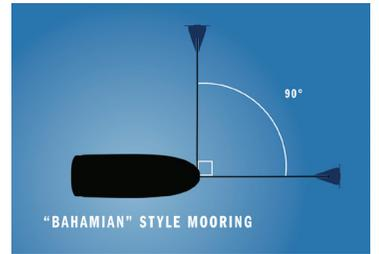
Any anchor can fail to reset once it has been pulled out of the sea bottom. Don't be fooled by some manufacturer's claims about an anchor's ability to dependably reset 100% of the time. Set two anchors if you expect a change in current or wind.
