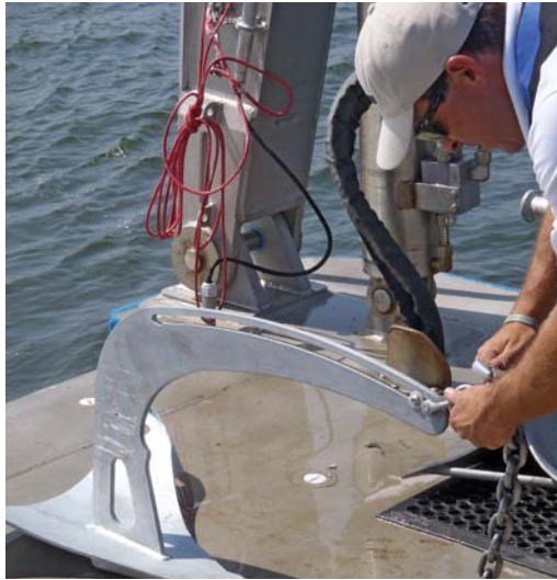
LEFT: Ocean Marketing's Jeff Cox chats with Chuck Hawley (red hat) during testing; and inspects the chain connection on the Manson Boss anchor.
