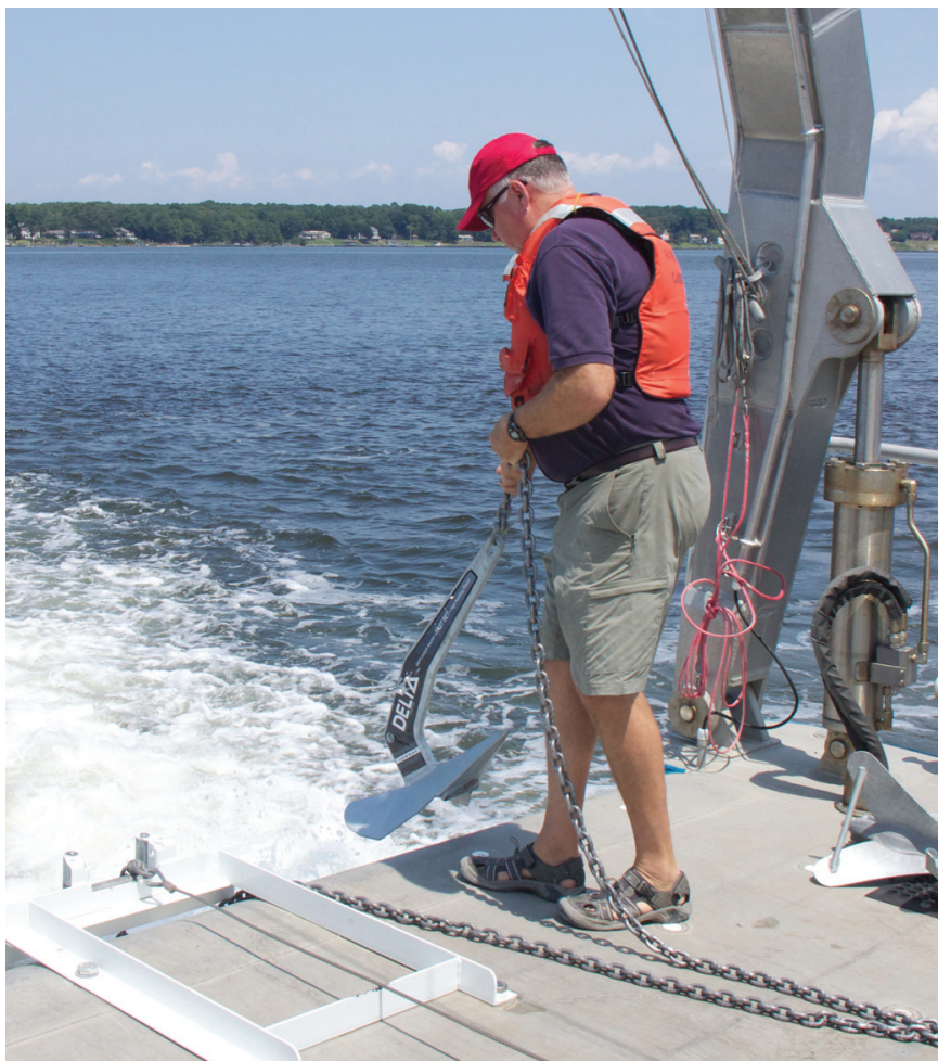
Chuck Hawley, acting as an independent reviewer, deploys a Delta anchor for testing. Each anchor was deployed and tested five different times in five unique locations.
