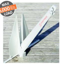
a fluke slightly during our veering test. This was while the anchor was under load, so it would be unfair to say anything other than it withstood a tremendous amount of abuse and still functioned properly. It would be difficult (but not impossible) to secure in a bow roller when not in use.
